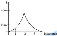
The ball reaches the ground when x = 19.6 m. This gives t = 2s. After that it moves up, x decreases and at t = 4s, x becomes zero, the ball reaching the initial point.
