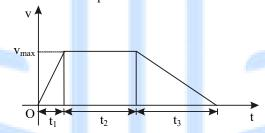
$$\therefore S = \frac{v_{max}t_1}{2}$$
